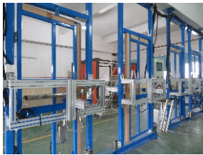
Test devices for exit devices, door coordinators
