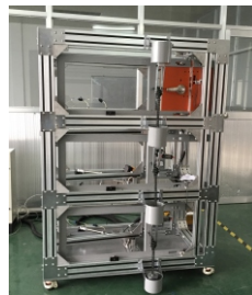
Test devices for ANSI/Euro mortise locks
