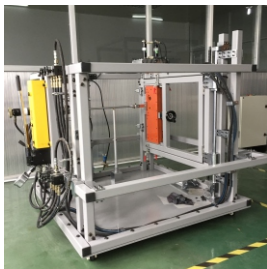
Test devices for ANSI/Euro mortise locks
